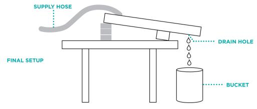
Place the bucket under the drain hole. You will need to empty the bucket periodically. Try to pour out just the water from the bucket, leaving behind any sand that has flowed out the drain.
