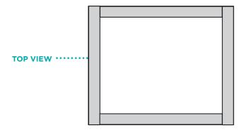
Turn the table over so that the two-by-fours are on the bottom. Nail the 10-cm two-by-fours to the underside of the table. They should be on the same side as the drain hole, but about 20-30 cm closer to the center of the table. See the diagram below. This will allow the drain hole to stick out over the end of the support table.
